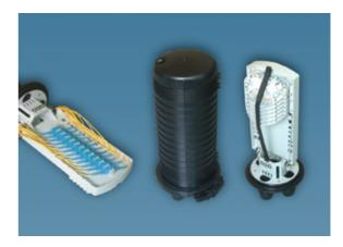
It accommodates up to 20 splice trays. Its adapter mount can equip 24 SC, FC or LC adapters. It also supports 2 splitters for fiber optic service drops in FTTX deployment. Air valve is available as an optional accessory.
