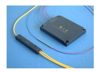
1xN tree couplers and NxN star couplers are made with fuse cascade-connecting (N-1) pieces of 1x2 and 2x2 couplers respectively.
